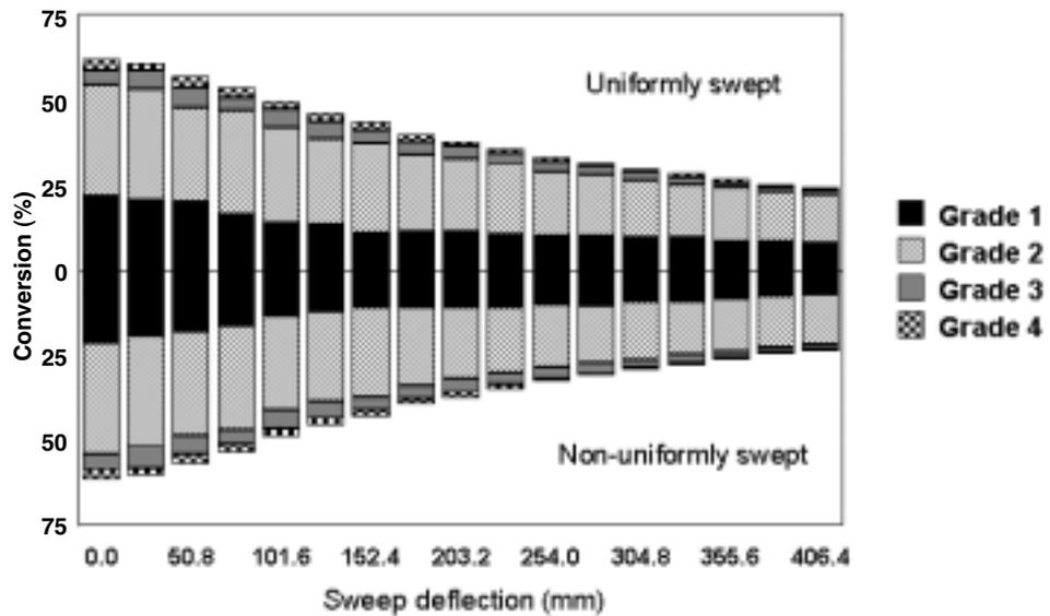
FIG. 7–Comparison of grade distributions from uniformly and non-uniformly swept logs.
