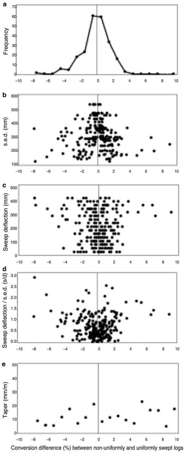
FIG. 5a–e: Conversion differences and characteristics of the 120 paired logs (bent at quarter- and half-way along the log) for which differences were recorded.
