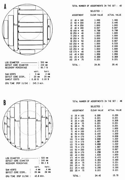
FIG. 2A—Optimisation by value with vertical saw kerf size at 3 mm. B—Optimisation by volume.
