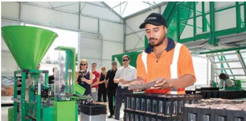
*Nursery Technician Ngarimu Mana demonstrating paper pot production, for seedling and cutting propagation, using an Ellepot production line. Scion has the machine on loan for research trials, and significant industry interest in the technology has resulted.*
