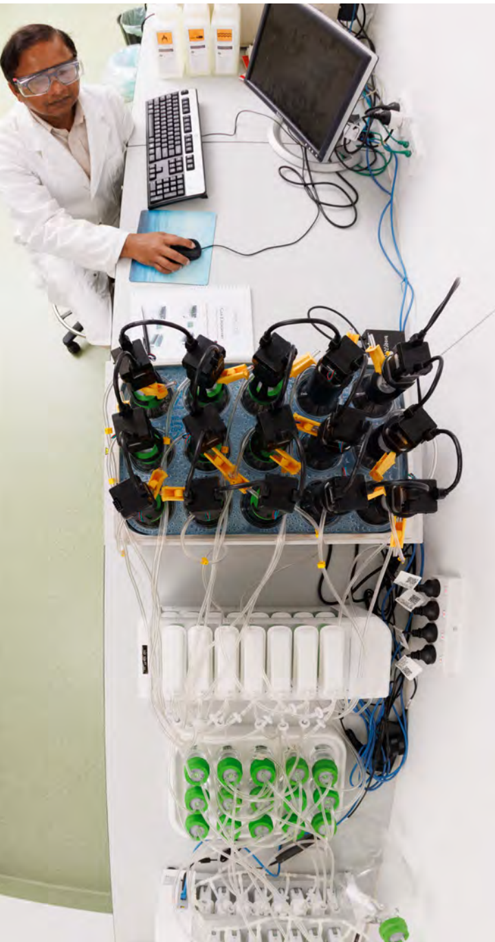
Dr Suren Wijeyekoon uses the biomethane potential test kit during the first stage of research.
