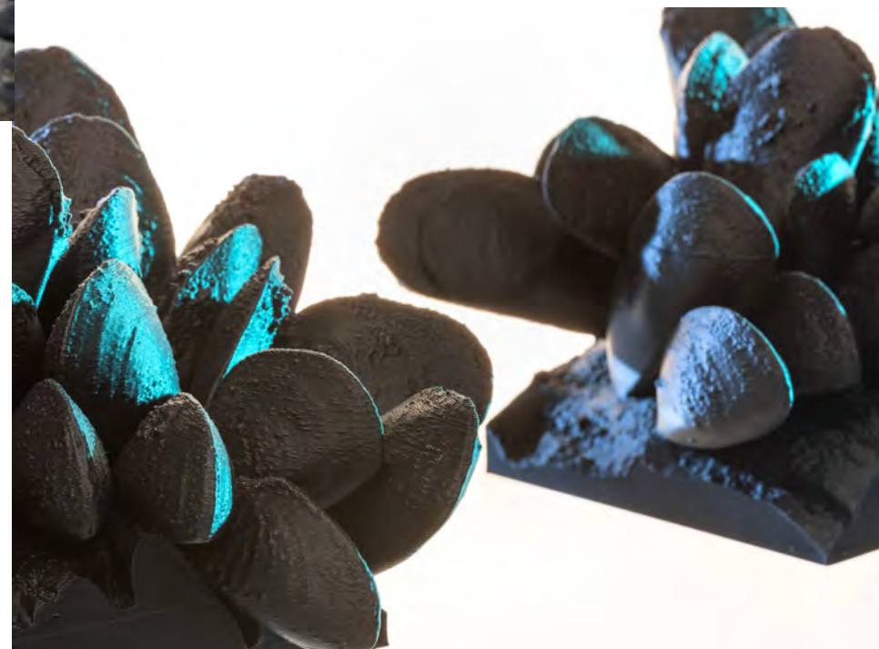
Mussel substrates recreated in the 3D printing lab.
