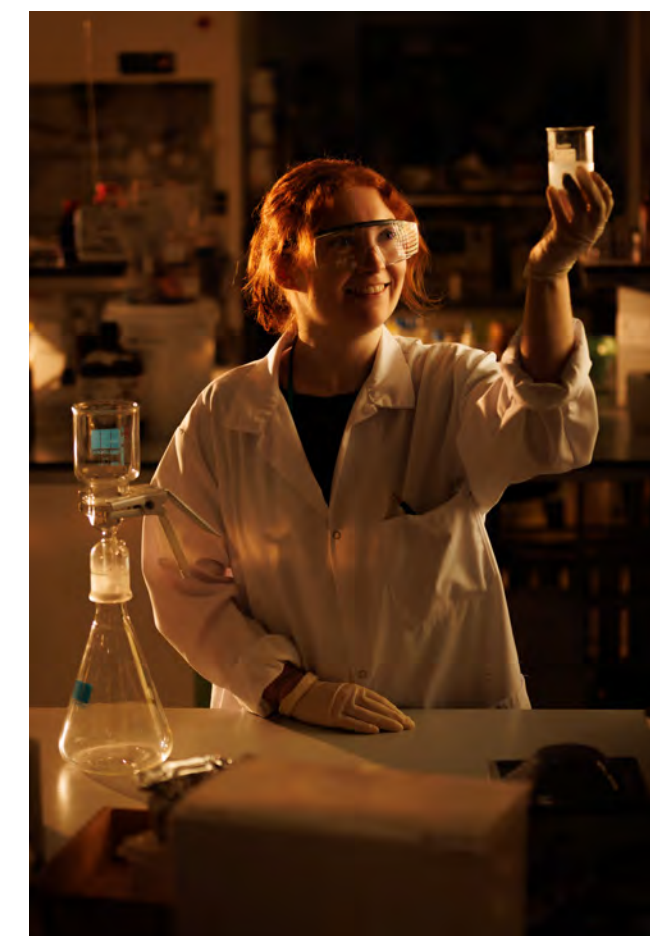
Janet Reid using a vacuum filtration setup to apply a layer of nanocellulose to a paper scaffold.
