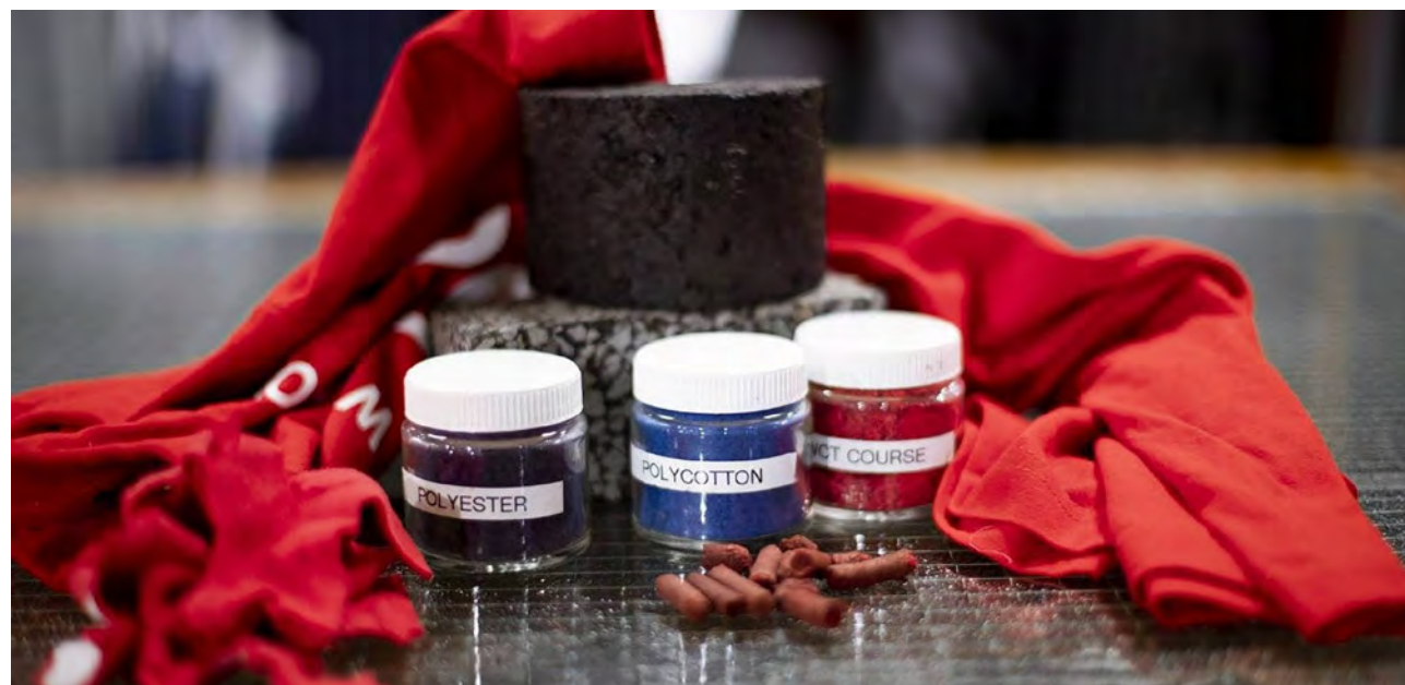
Scion is supporting UsedFULLY with technology that can turn unwanted textiles into an ingredient used to create New Zealand roads.
