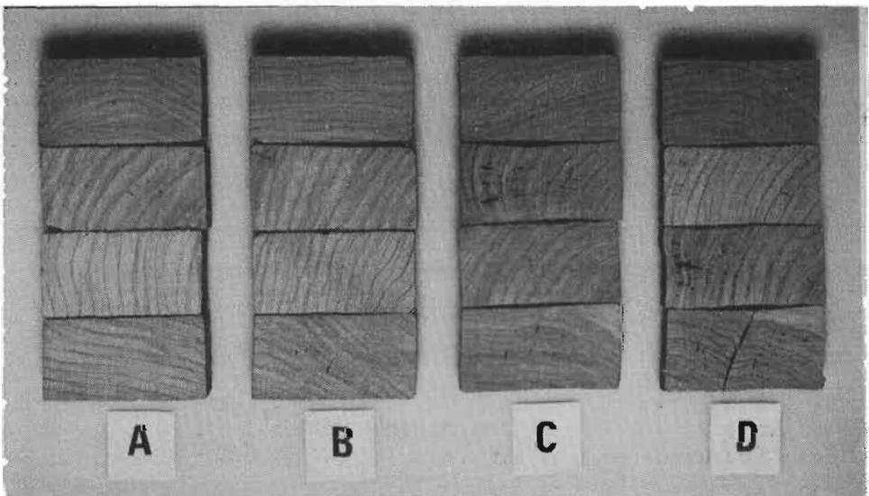
FIG. 1—Matched cross-sections of *Cupressus macrocarpa* showing increased degrade with increased severity of drying conditions: A - air drying; B - 38°/35°C to 38°/30°C; C - 54°/51°C to 65.5°/54.5°C; D - 71°/60°C.
