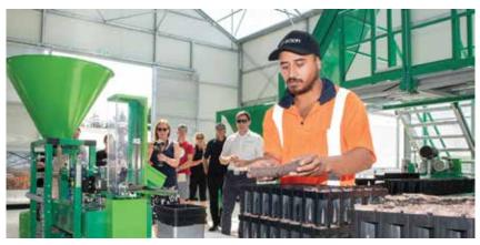
Nursery Technician Ngarimu Mana demonstrating paper pot production, for seedling and cutting propagation, using an Ellepot production line. Scion has the machine on loan for research trials, and significant industry interest in the technology has resulted.
