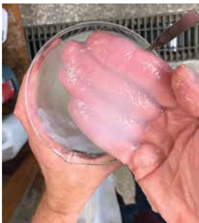
Jelly-like seaweed-based nanocellulose hydrogel.
