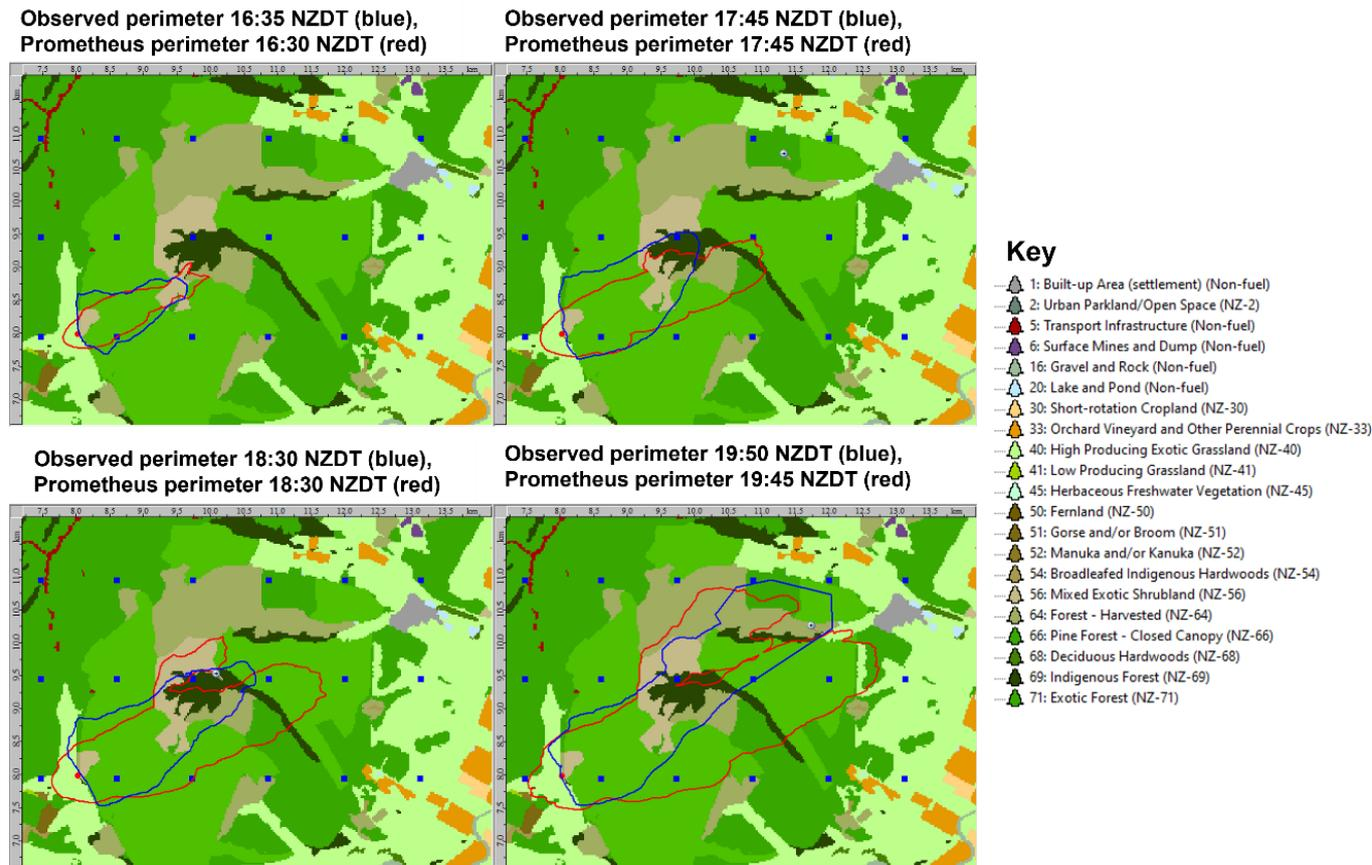
Figure A1: Run 5 modelled (red outline) and actual (blue outline) fire perimeters for 16:30 to 19:50 NZDT on 5 February 2019. The Virtual weather stations from the NZCSM gridded meteorological data is depicted as blue squares. Modelled fuel types are shown in the background and were obtained from data provided by Tasman Pine Forest Ltd.
