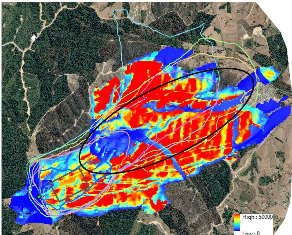
Figure 7: Run 5 modelled fire intensity (kW/m) shown in colours ranging from blue (low values) to red (high values). The actual/observed hourly fire perimeters between 16:30 and 21:40 are shown for spatial context.
