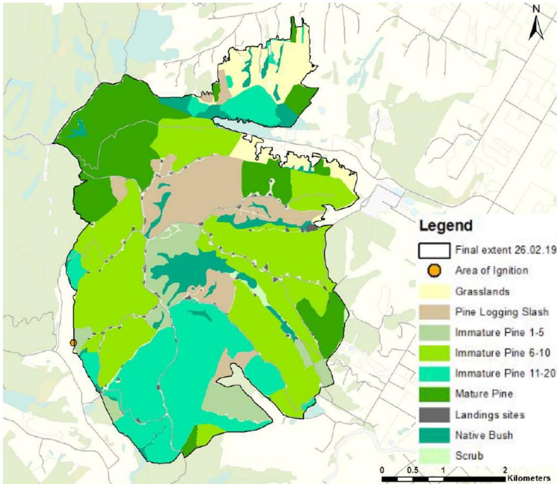
Figure 3: Fuels distribution within the Pigeon Valley fire final perimeter. Data sourced from Tasman Pine Forest Ltd. Image adapted from Clifford 2019.
