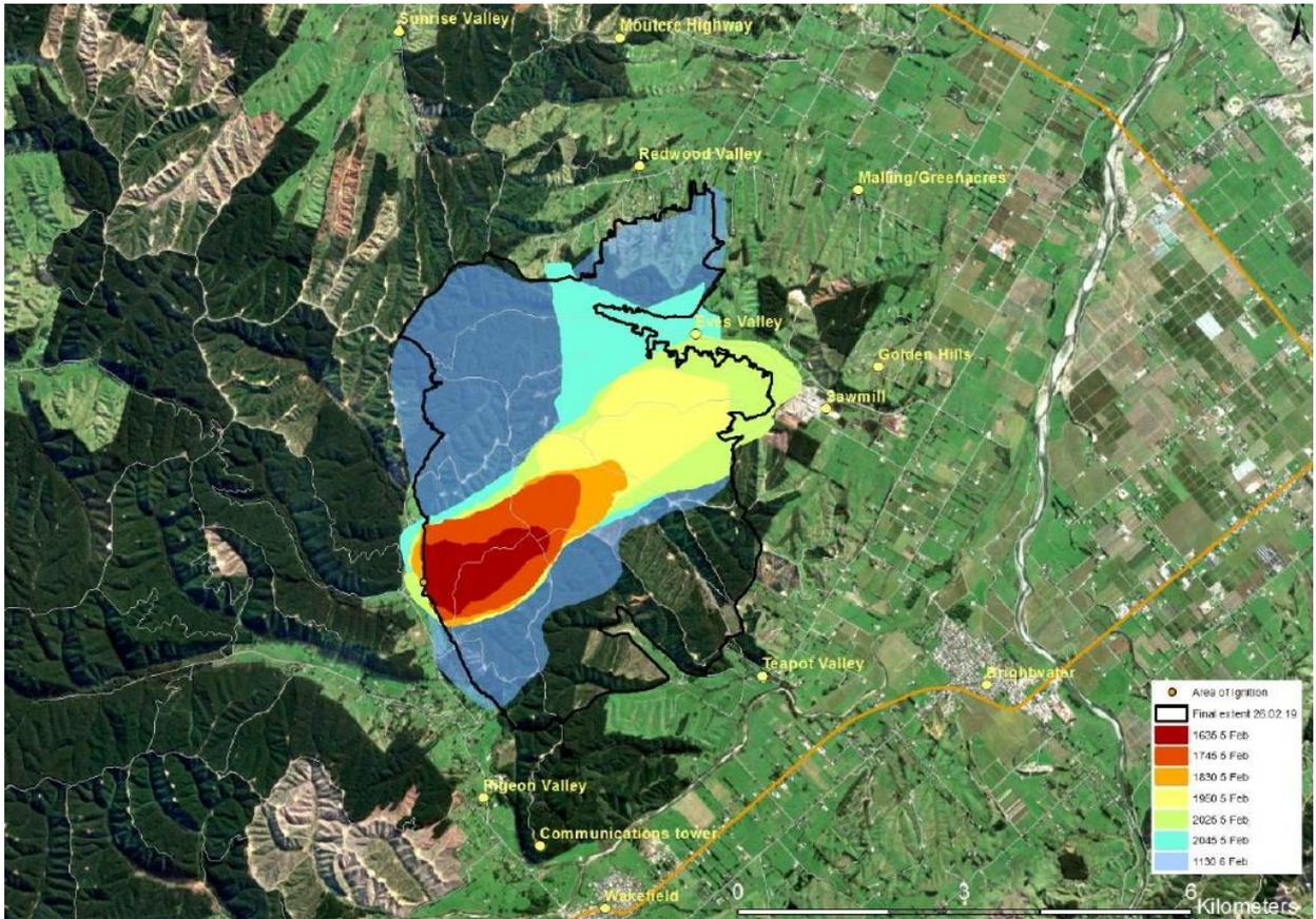
Figure 1: Estimated progression of the Pigeon Valley fire on the first and second days. The final estimated perimeter is outlined in black (retrieved from Clifford 2019).
