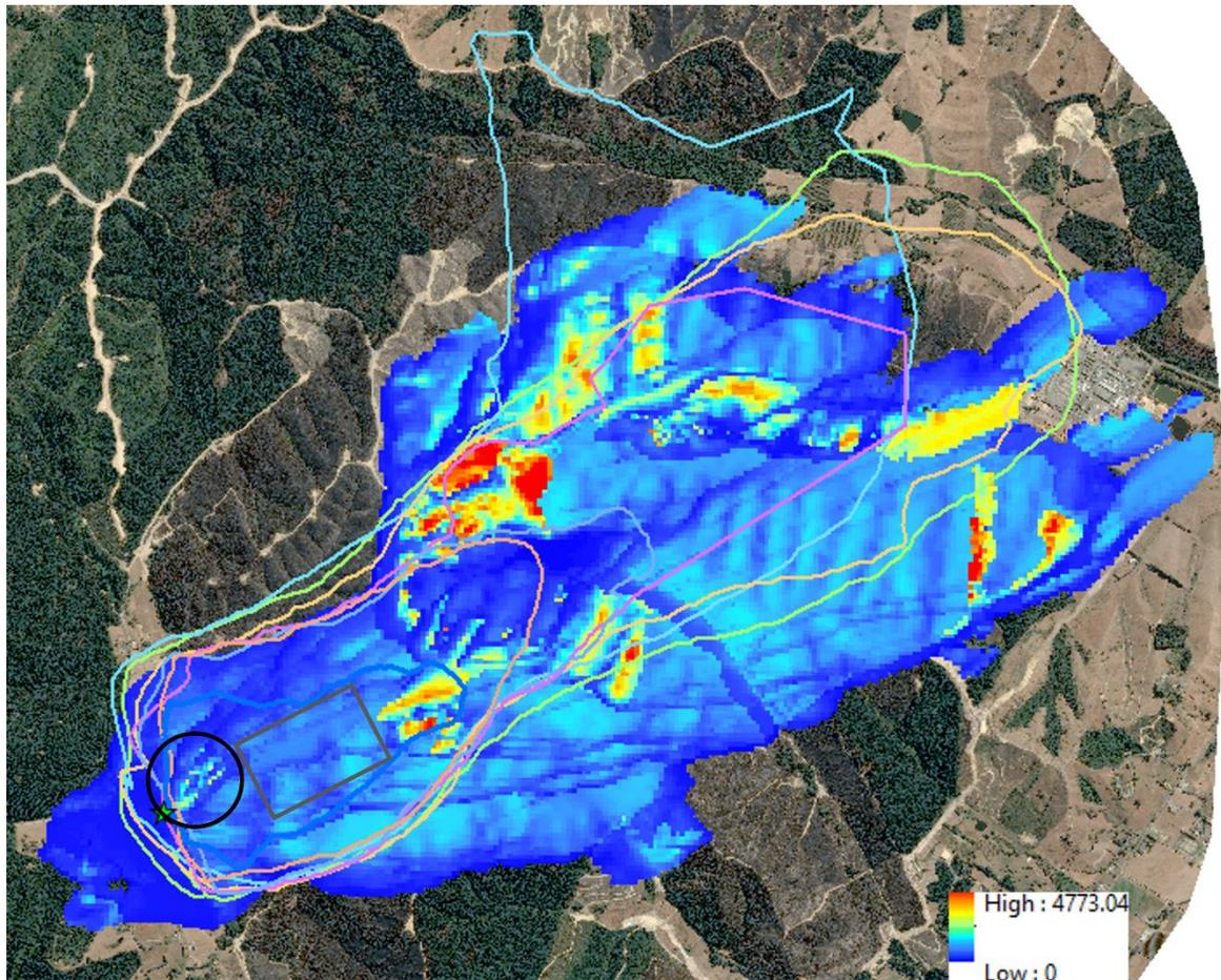
Figure 5: Run 5 modelled Rate of Spread (ROS) (m/h) shown in solid colours ranging from blue (low values) to red (high values). The actual/observed hourly fire perimeters (lines) between 16:30 and 21:40 are shown for spatial context.
