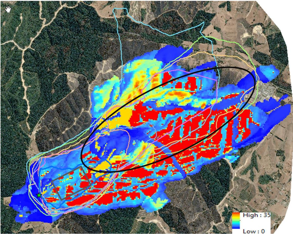
Figure 6: Run 5 modelled flame lengths (m) shown in solid colours ranging from blue (low values) to red (high values). The actual/observed hourly fire perimeters (lines) between 16:30 and 21:40 are shown for spatial context.
