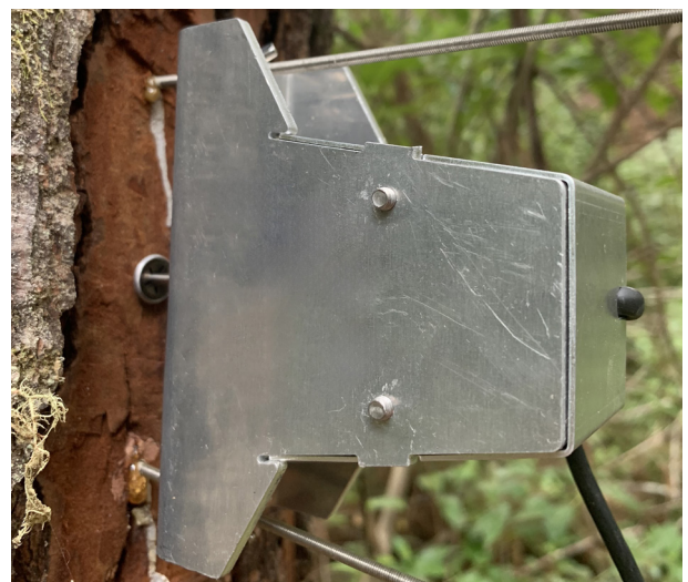
Smart dendrometer measures tree growth and water use.
