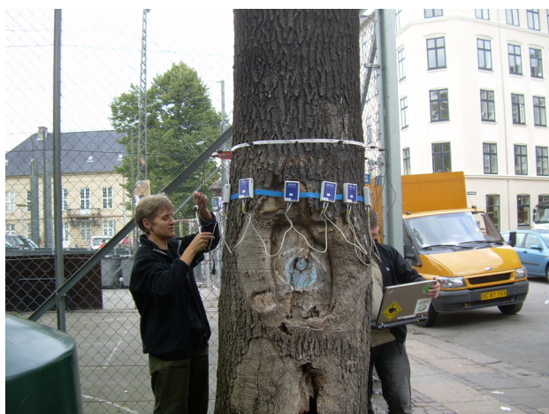
Iben Thomsen (left) and colleague using the Picus to look for decay in an urban tree in Copenhagen, Denmark.
