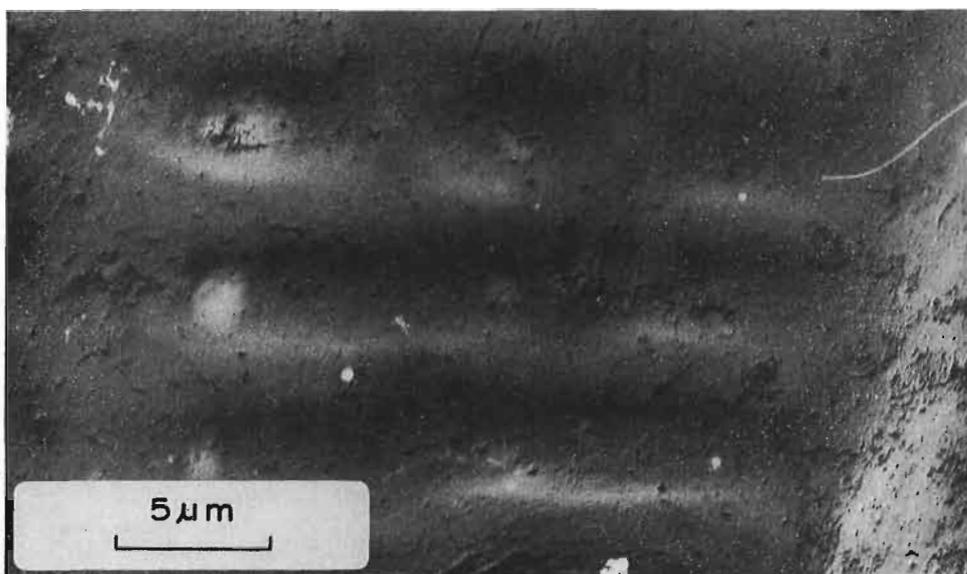
FIG. 3—Area of vessel/ray (scalariform) pits completely occluded in unsteamed control.
