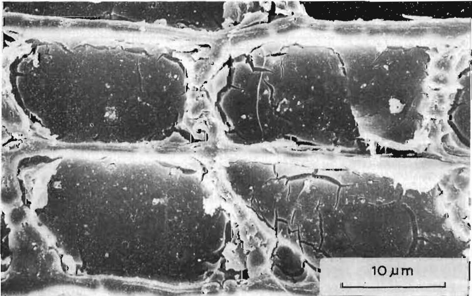
FIG. 14—Appearance of a radial section without steaming showing a denser and relatively uniform lining of the lumen surface. Cracking was probably caused by drying.
