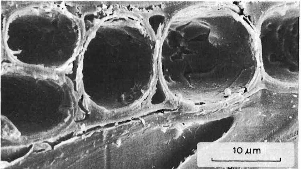
FIG. 11—Appearance of a control wood ray in a scanning electron microscope.
