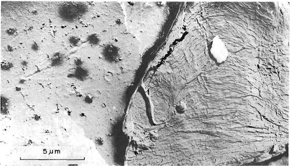
FIG. 9—Ray parenchyma lumen showing the lining of these surfaces in unsteamed material.
