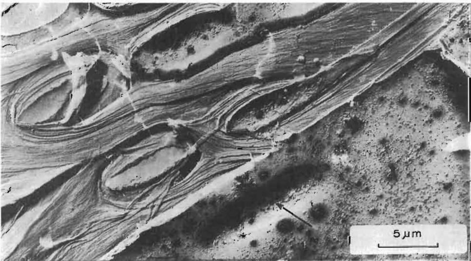
FIG. 2—Heavy deposit lining a vessel lumen, covering a vessel/ray-pit aperture (1) and adhering to a pit membrane (2).
