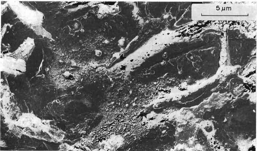
FIG. 6—General area of pits in steamed heartwood in which the coating materials have tended to flow.
