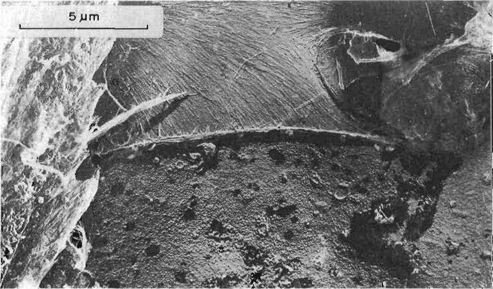
FIG. 1—Replica of a vessel wall with the wall layers exposed where the encrusting material, possibly in a tylosis, has been torn in preparation.
