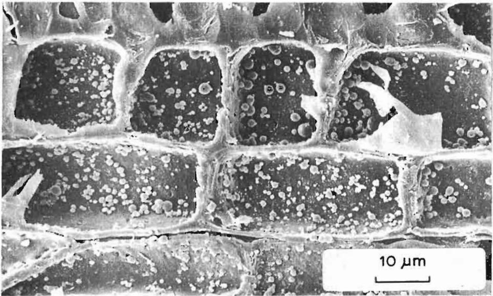
FIG. 13—Radial section of a wood ray of steamed material viewed in a scanning electron microscope. Material steamed at 115°C in a pressure vessel.
