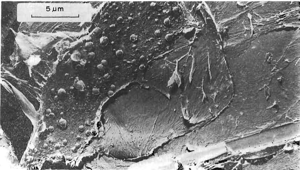
FIG. 10—Lumen surface of a steamed ray cell in which the occluding material has become discontinuous, forming rounded bodies.
