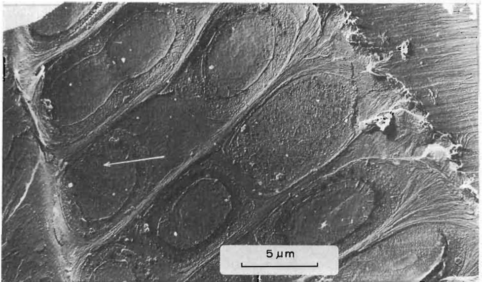
FIG. 7—Area of vessel/vessel pit membranes in unsteamed material. Pit membranes appear to be slightly occluded and overlain by an extra layer which has folded back (see arrow) during preparation.
