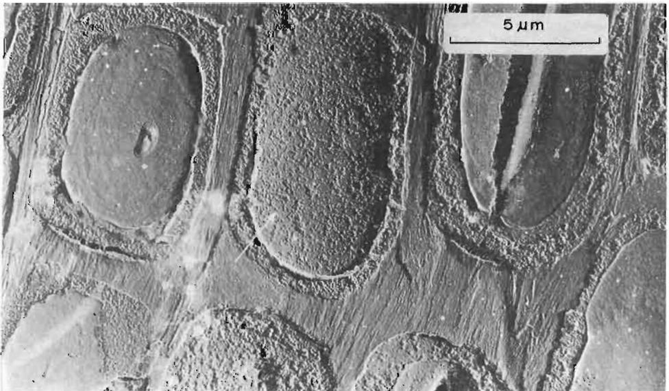
FIG. 8—An area similar to Fig. 7, after steaming. The extra layer over the pit membrane is modified in one case (arrowed) but not in others and the material forming the primary occlusion of the pit membrane has broken up into rounded areas.
