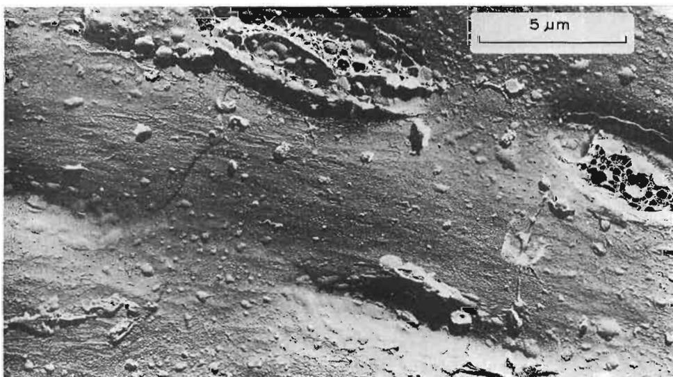
FIG. 4—Appearance of a vessel lumen in steamed heartwood. Coating material has broken down over some pit apertures and elsewhere it has blistered or formed rounded bodies.
