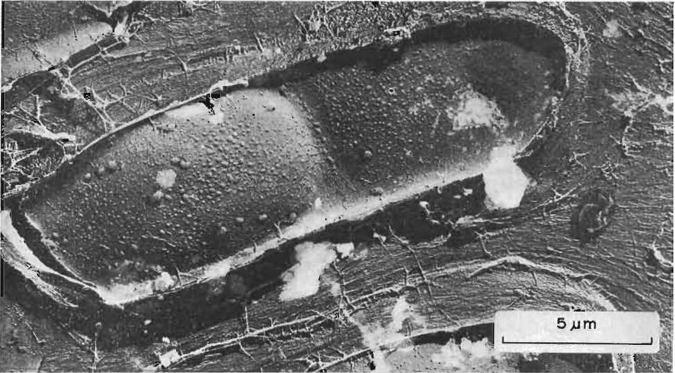
FIG. 5—Vessel/ray-pit membrane in steamed heartwood showing blistering of occluding deposits.
