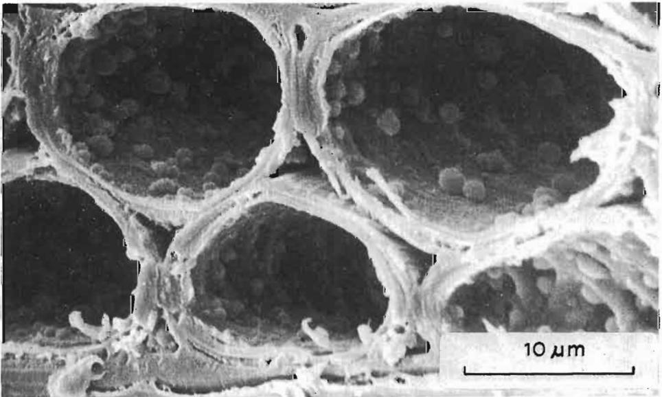
FIG. 12—View of a tangential section similar to Fig. 11, after steaming, showing the characteristic change in appearance of material occluding the lumen surface.
