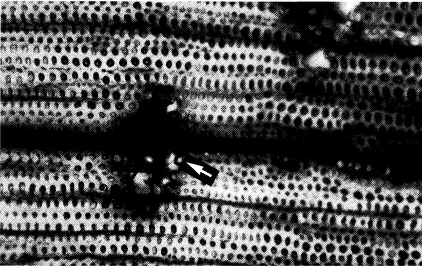
FIG. 5—Intersection of a radial and an axial resin canal in transverse section
