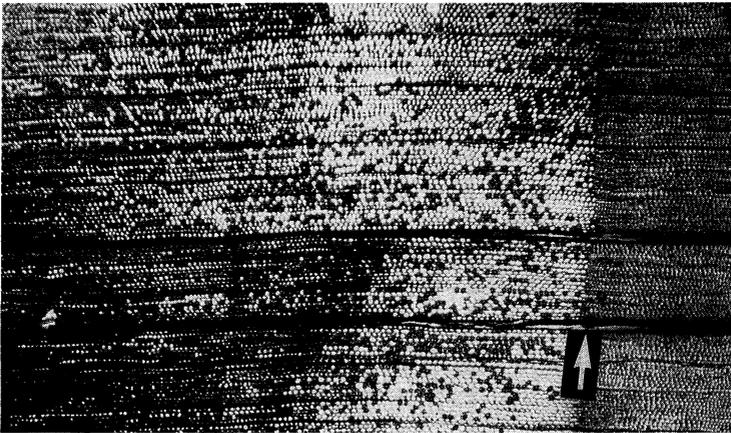
FIG. 7—Two conducting radial resin canals passing through both earlywood and latewood. A stained axial resin canal (arrowed) is visible near the earlywood to latewood boundary
