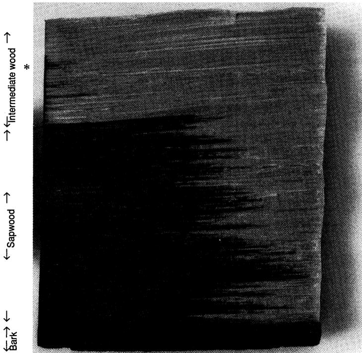
FIG. 1—Dye-flow through a green rimu specimen cut from baulk 48A 100 mm along the grain direction. The direction of flow is from left to right. The penetration of the intermediate wood is very small compared to that of the sapwood. The boundary between sapwood and intermediate wood was recorded before the dye penetration experiment.
