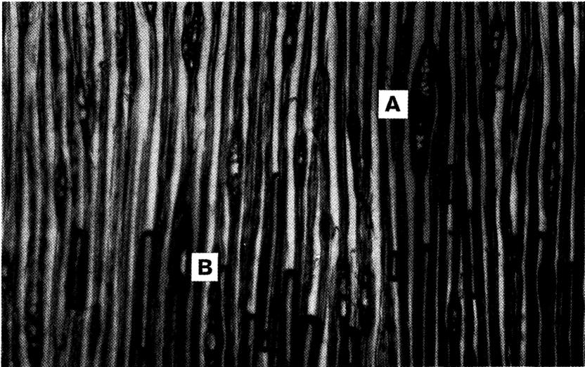
FIG. 6—Radial dyeflow seen in tangential-longitudinal section
