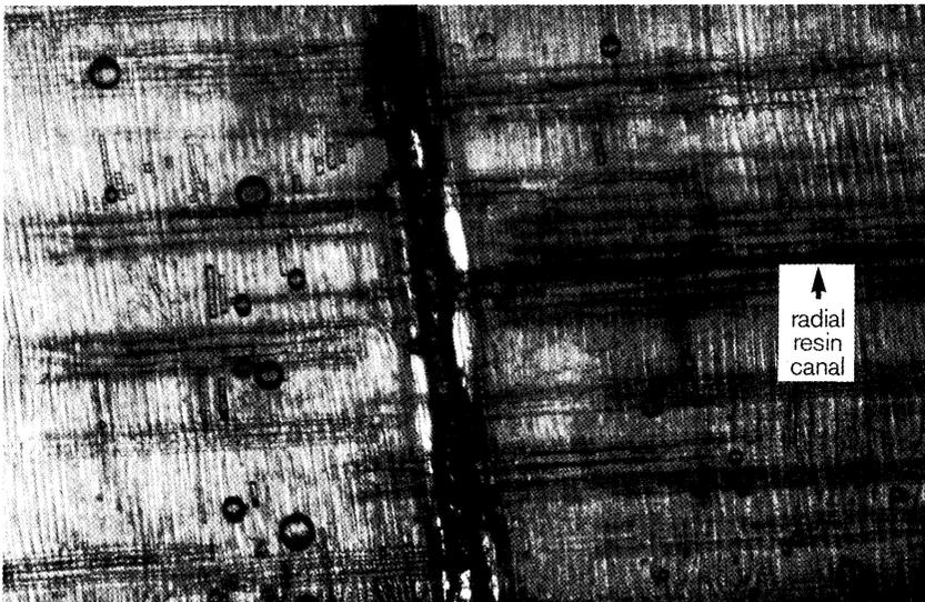
FIG. 3—Enlargement of the intersection of the radial and axial resin canals in Fig. 2
