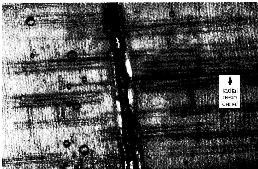
FIG. 3—Enlargement of the intersection of the radial and axial resin canals in Fig. 2
