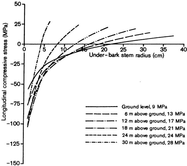
FIG. 3 — Longitudinal growth stress gradients at 6-m height intervals in 75-cm dbhob *E. regnans* by height, based on 9 MPa peripheral stress at ground level (after Kubler 1959).
