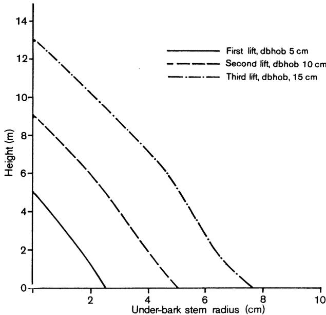
FIG. 2 — Under-bark taper of *E. regnans* by pruning lift (after Hayward 1987).
