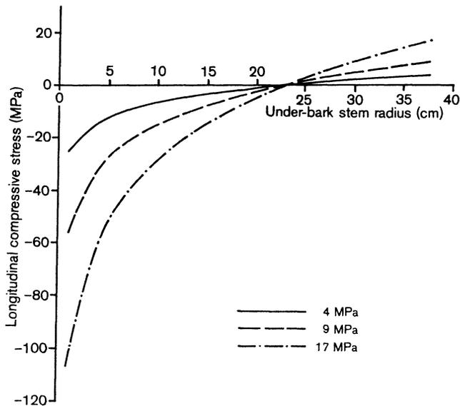
FIG. 4 — Longitudinal growth stress gradients at ground level in 75-cm dbhob *E. regnans* for 4-, 9-, and 17-MPa peripheral stress values (after Kubler 1959).
