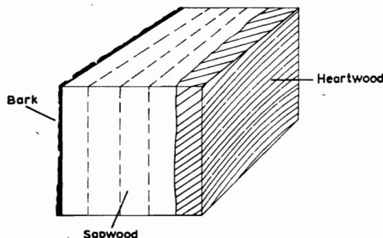
FIG. 1—Dissection of groups into slabs. The broken lines show how the sapwood was split into slabs.
