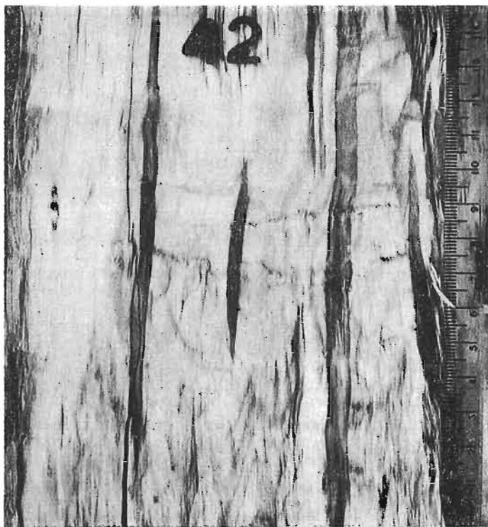
FIG. 3—A group in Experiment 2 at 10 mm into the sapwood, showing faint stain around the aseptically-drilled hole. Left to right—aseptically-drilled hole, *Ceratocystis*-inoculated hole, *E. platypodis*-inoculated hole, Fungus A-inoculated hole, open hole. Note that the stain below the open hole is partly obscured by shadow and the stain below the hole inoculated with Fungus A runs off the slab.
