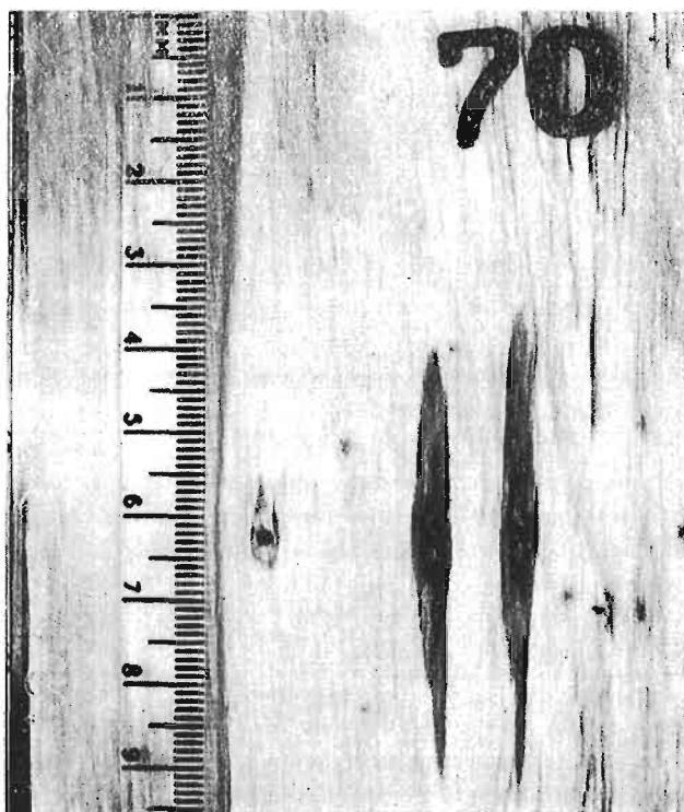
FIG. 2—A group in Experiment 1 at 18 mm into the sapwood, showing faint stain around the aseptically-drilled hole. Left to right—aseptically-drilled hole, inoculated hole, open hole.
