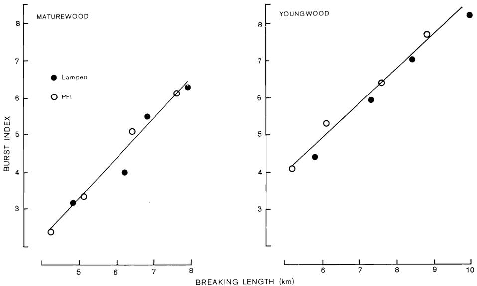
FIG. 5—Laboratory radiata pine kraft (Kibblewhite, 1973) — burst and breaking length.
