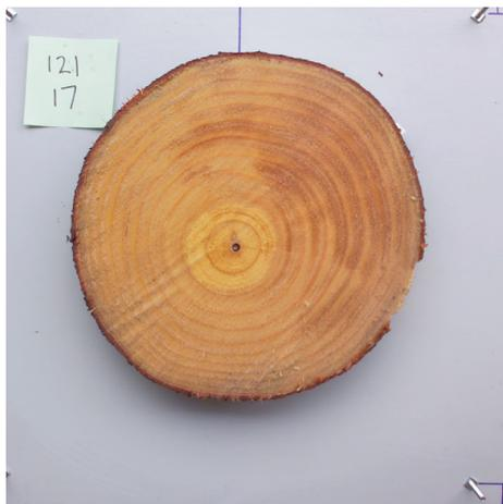
FIG. 1—Image of sample disc 121/17 on the reference frame. Four pins extending 50 mm above the frame surface were located at the corners of a square of known dimension (500 mm) to establish a measurement plane.
