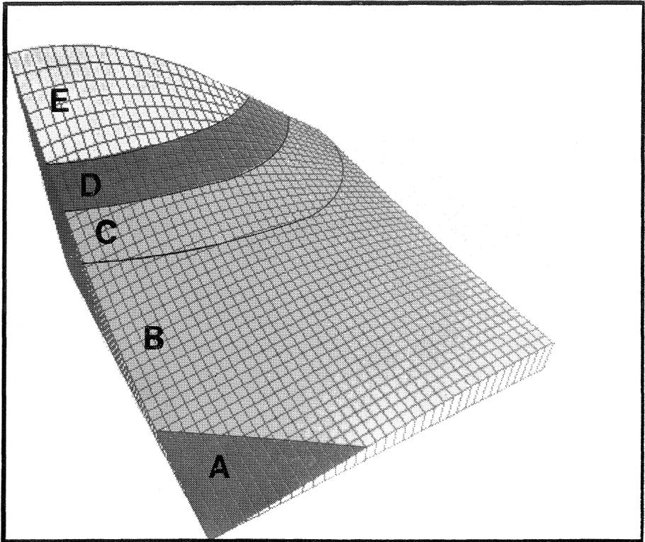
FIG. 4.—Energy ratio surface during platen pressing of *Eucalyptus regnans*: effect of changes in initial degree of pore saturation and strain.
