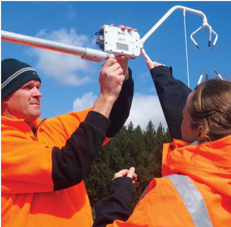
Liam Wright and Dr Christina Dunker install a sonic anemometer.
