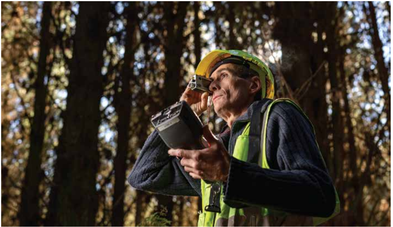
Stephen Pearce takes tree measurements using a Haglöf vertex and enters the data into an Allegro data manager.
