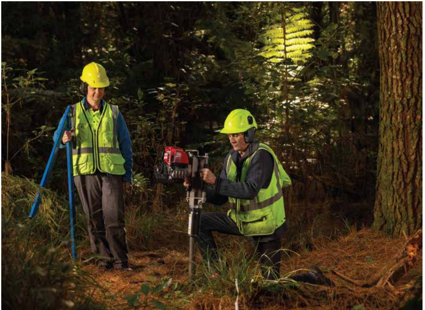
Soil percussion auger – taking an intact soil core down to 1 metre, which tells us the nutrient stocks on site in the soil.
