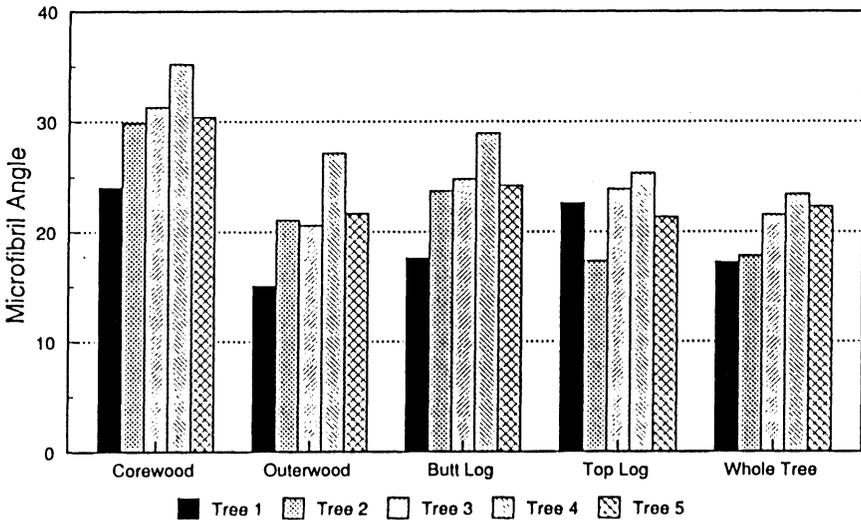
FIG. 4—A comparison of volume-weighted microfibril angle among trees for corewood and outerwood at breast height, the butt log (0–7 m), the top log (23–30 m), and the whole tree.
