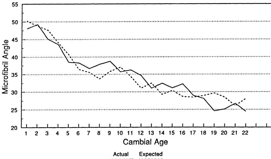
FIG. 6—Predicted and actual mean microfibril angles at the butt, based on mean microfibril angles measured at breast height.
