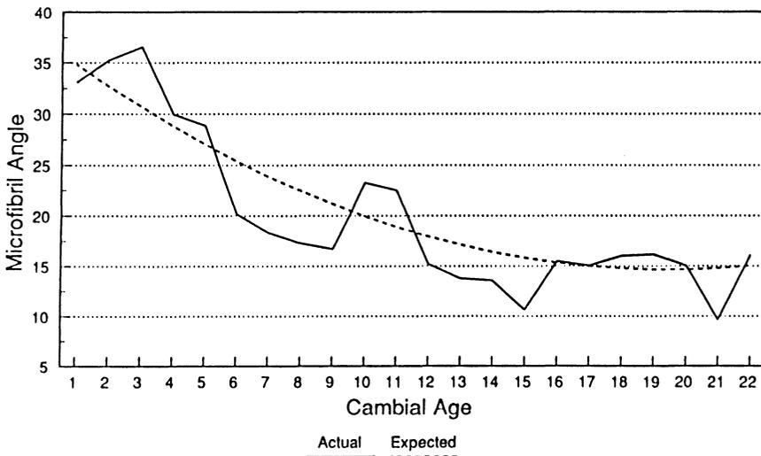
FIG. 5—Predicted and actual microfibril angle for Tree 1 at breast height based on a regression between microfibril angle and cambial age using rings 1, 5, 10, 15, 20, and 22.
