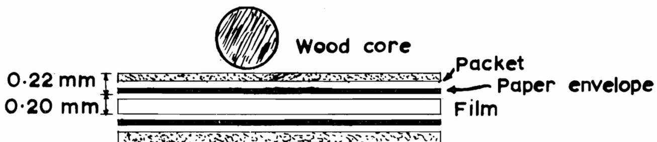
FIG. 2—Cross section of Kodak X-ray film in the envelope and packet, with a wood core resting on it.
