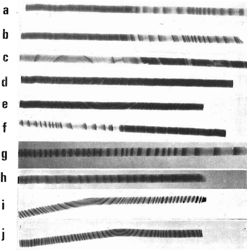
FIG. 3—The effect of the position of the cores and their moisture content on the quality of the radiograph.
