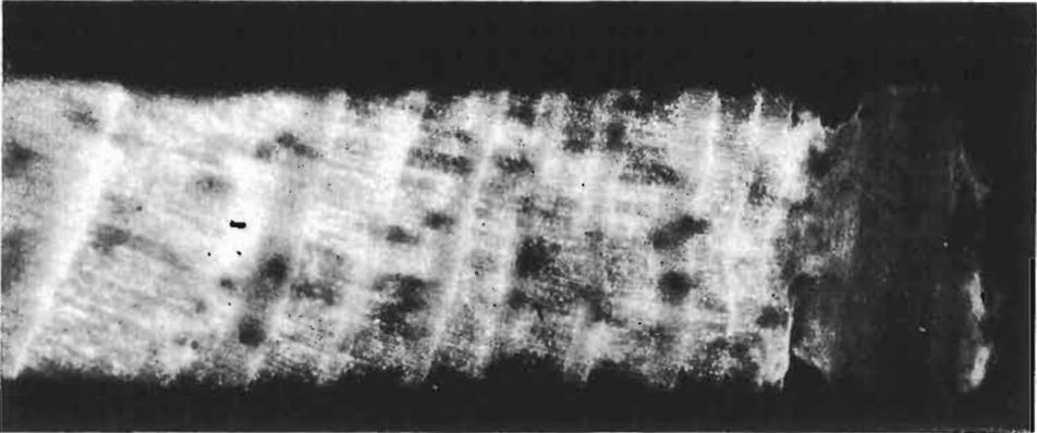
FIG. 4—Radiograph of part of a *Pinus ponderosa* core magnified seven times (dosage 25 kV, 300mA, 1.2sec.; light areas show greater X-ray absorption).
