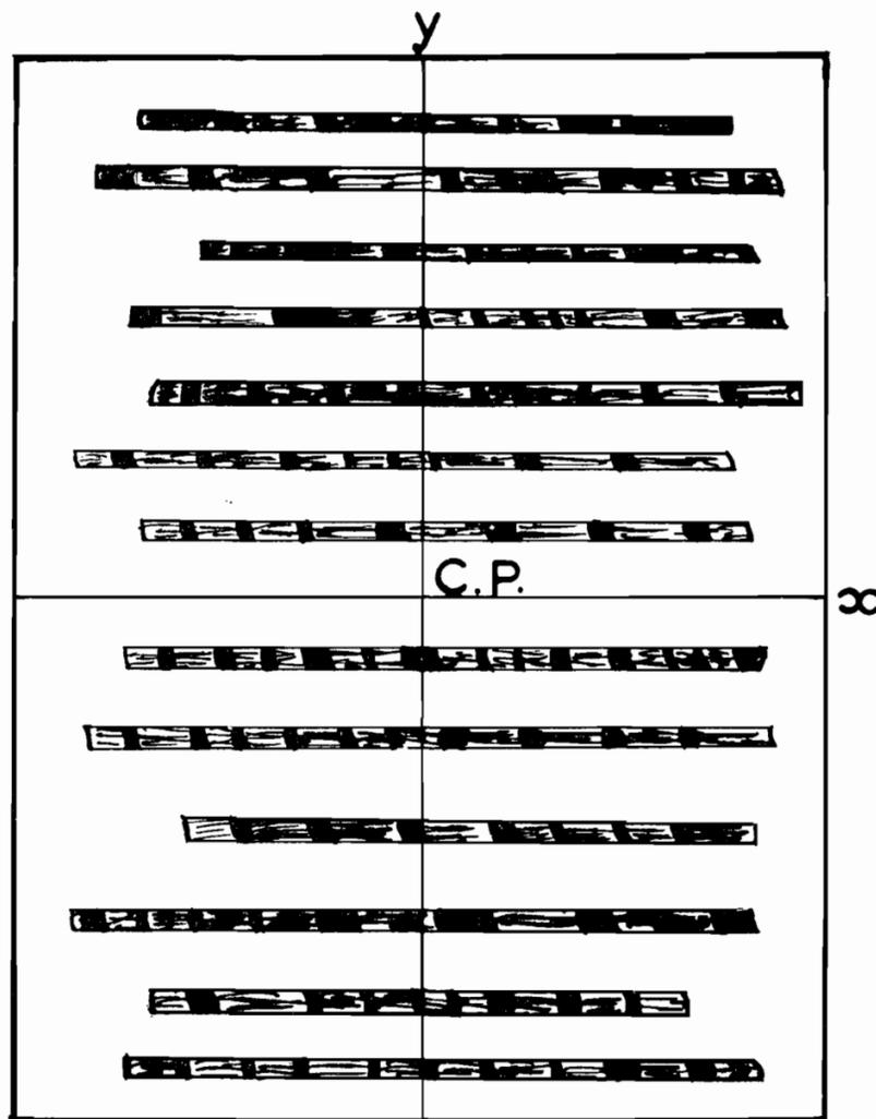
FIG. 1—Cores arranged on upper side of Kodak X-ray film (204mm × 254mm).
