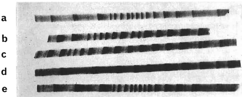
FIG. 5—Radiographs of *Pinus radiata* cores infused with Urografin, 25kV, 300mA, 1.0sec. dark areas show greater X-ray absorption. The dark latewood bands are extended to the right by the compression wood. The core in Fig. 5d was not taken at right angles to the main axis of the stem.
