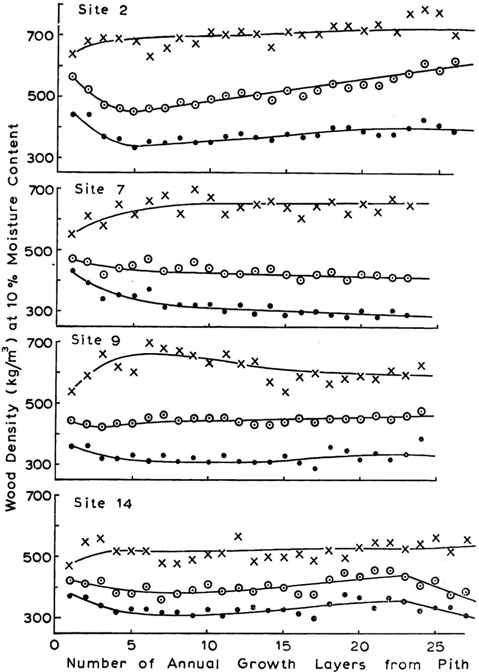
FIG. 3—Radial patterns of (methanol extracted) wood density variation on four sites planted with the "green" strain of lodgepole pine from Cpt 2 Waitapu Forest. The upper line of each set represents maximum density, the centre line mean density, and the lower line minimum density of each growth layer: average values for five trees on each site.
