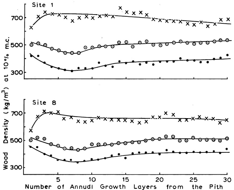
FIG. 4—Radial patterns of (methanol extracted) wood density variation on two sites planted with the Manning “green” strain of lodgepole pine. The upper line of each set represents maximum density, the centre line mean density, and the lower line minimum density of each growth layer: average values for five trees on each site.
