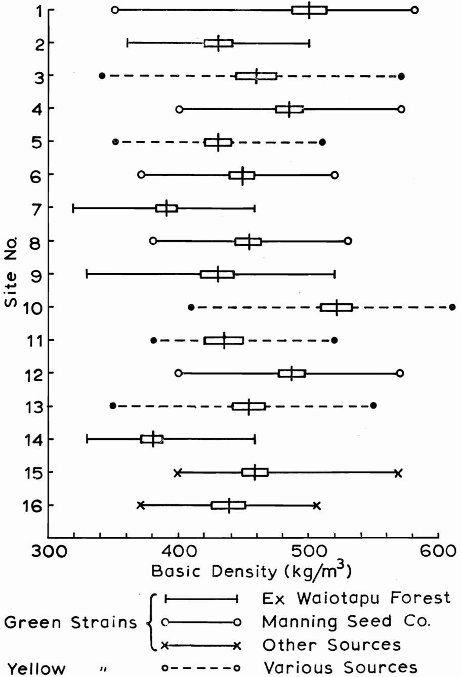
FIG. 1—Range of wood density of the outer 10 growth layers at breast height for each site. Each vertical line is at the mean value: the boxes represent two standard errors on either side of mean values.
