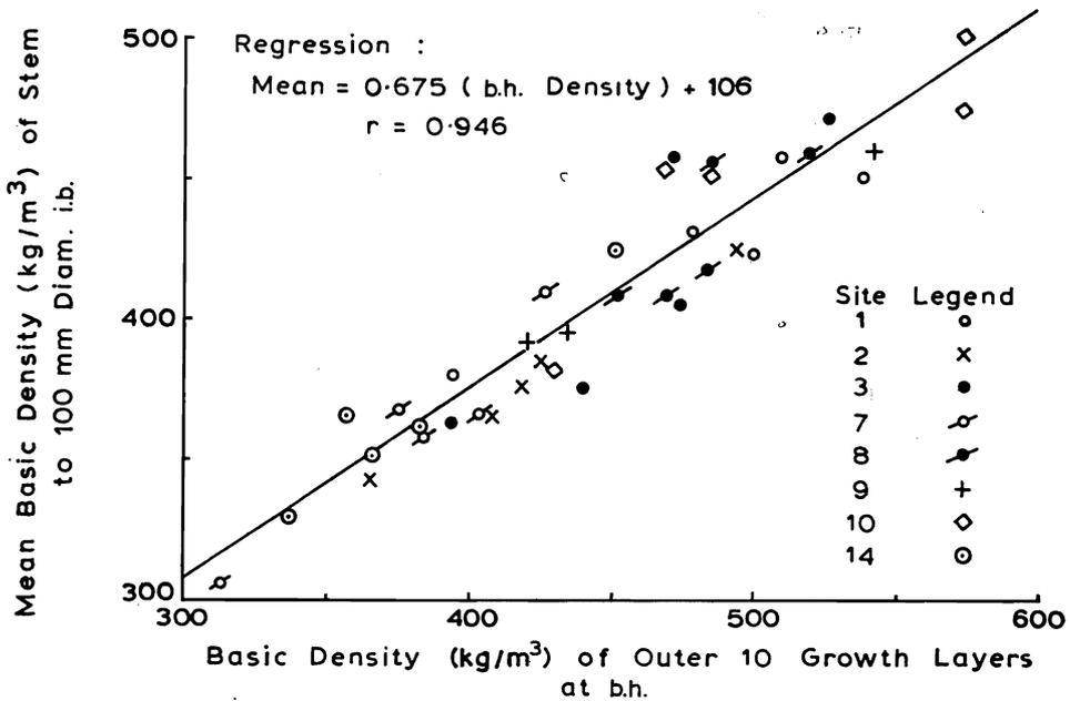
FIG. 2—Relationship between density of the 10 outer growth layers at breast height and weighted average density of the merchantable stem to 100 mm diameter i.b.
