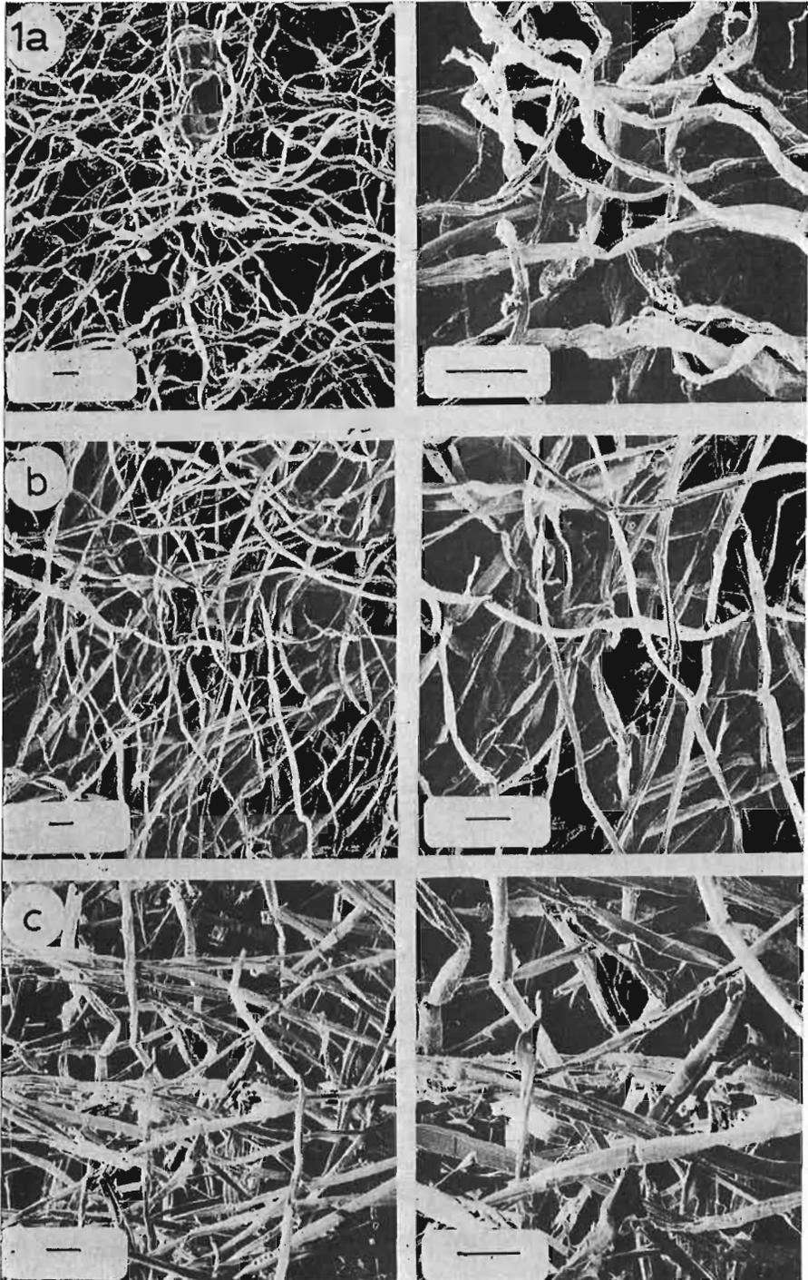
FIG. 1—Surface views of unbeaten latewood fibres in wet webs at 31.2% solids. Scale is 100  $\mu\text{m}$ .
