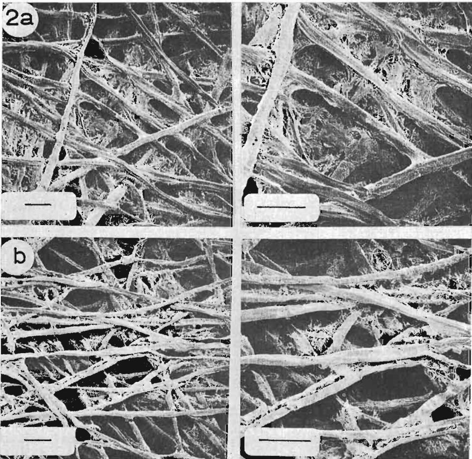
FIG. 2—Surface views of beaten (15,000 rev) latewood fibres in wet webs at 23.1% solids. Scale is 100  $\mu\text{m}$ .
