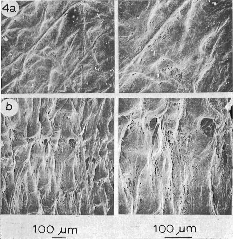
FIG. 4—Surface views of heavily beaten (55,000 rev) latewood fibres in wet webs at 22.7% solids.
