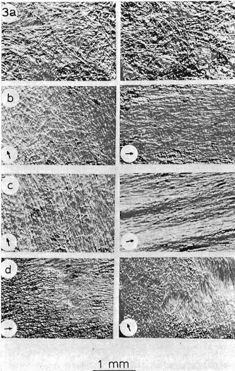
FIG. 3—Surface views of heavily beaten (55,000 rev) latewood fibres in wet webs at 22.7% solids. Micrograph pairs show a specimen under reflected light orientated parallel to, and perpendicular to, the direction of strain. Arrows indicate direction of web straining.
