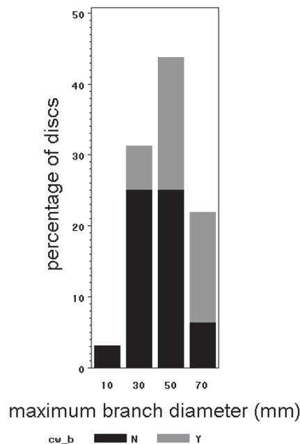
FIG. 6—Percentage discs below branch clusters that showed (cw\_b = Y) or did not show (cw\_b = N) signs of compression wood in relation to the diameter of the largest branch in the cluster immediately above the disc.
