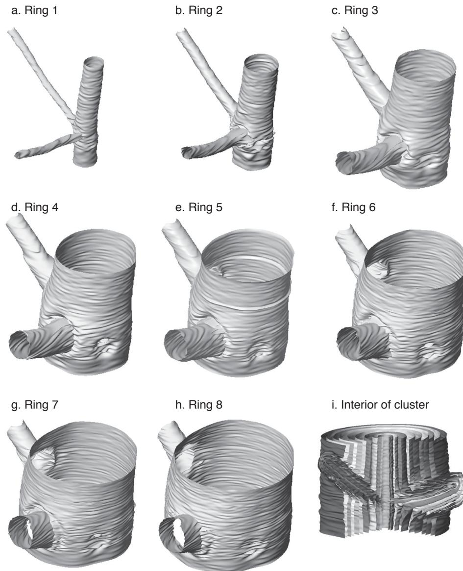
FIG. 2—Models showing the shape of each latewood band for growth rings 1 to 7 (a–g), stem edge (ring 8), and the complete cluster (i) with a wedge removed to show the interior of two branches. The exterior diameter of the cluster was approximately 190 mm.
