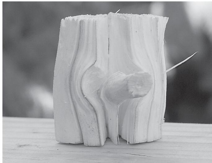
FIG. 1—Image showing delignified and separated stem-branch junction. The branch is 9 mm in diameter.
