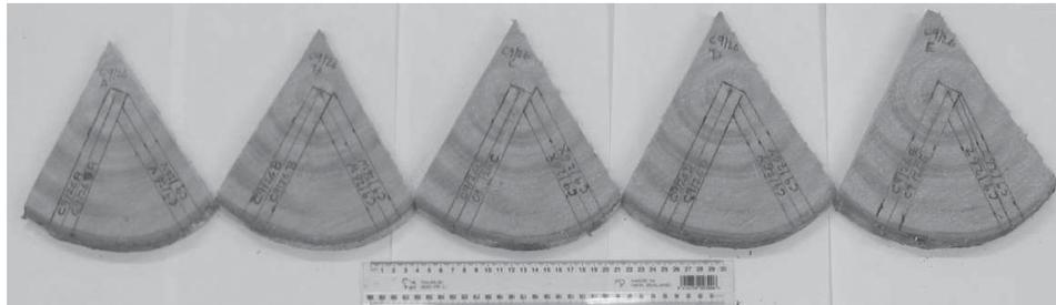
FIG. 3—Samples marked for SilviScan analysis from Tree C09. The left-hand slice was 2 cm below the base of the branch cluster. Each subsequent slice was 6 cm below the previous one. The two marked strips on each slice were analysed using SilviScan. Only one strip per slice included the stem pith.
