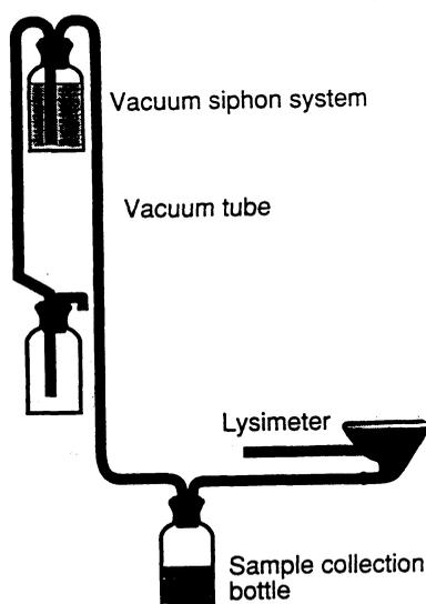
FIG. 2—Schematic representation of lysimeter system.
