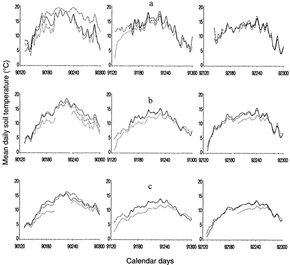
FIG. 4—Effects of harvesting methods on the daily mean temperature recorded at Depths 1 (a), 2 (b), and 3 (c) in control (.....), conventional (-----), and whole-tree (—) plots in Deersdale. The first two digits of the x-axis label refer to the year, the next three to the calendar day, i.e., 1 May = 120, 1 July = 182, 1 Nov. = 305.
