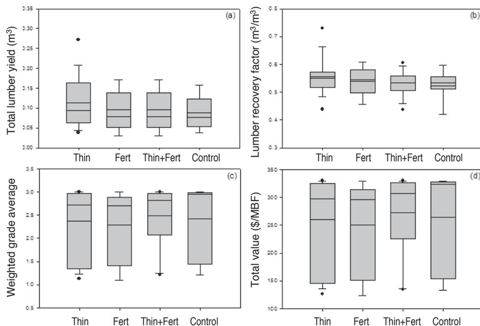
FIG. 3—Simulated lumber recovery by silvicultural treatment: (a) total lumber yield ( $m^3$ ); (b) lumber recovery factor ( $m^3/m^3$ ); (c) weighted grade average (Todoroki *et al.* 2005); and (d) estimated plot total log value (\$/MBF) from mean 2004 lumber prices.
