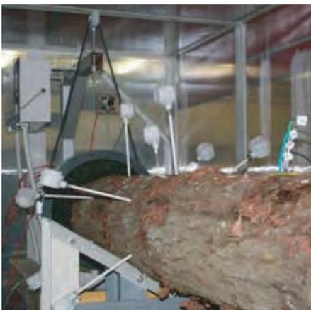
Laboratory rig showing a radiata pine log with temperature sensors inserted after Joule heating treatment.
