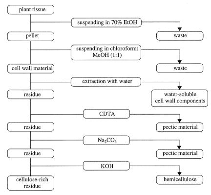
**B:** Extraction scheme for the preparation of carbohydrate oligomers for mass profiling
