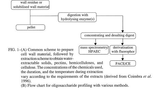
intact on the resulting oligosaccharides. Before characterisation of the polysaccharides can be performed, the enzymatic extracts are generally purified from salts by dialysis or ultra filtration.
