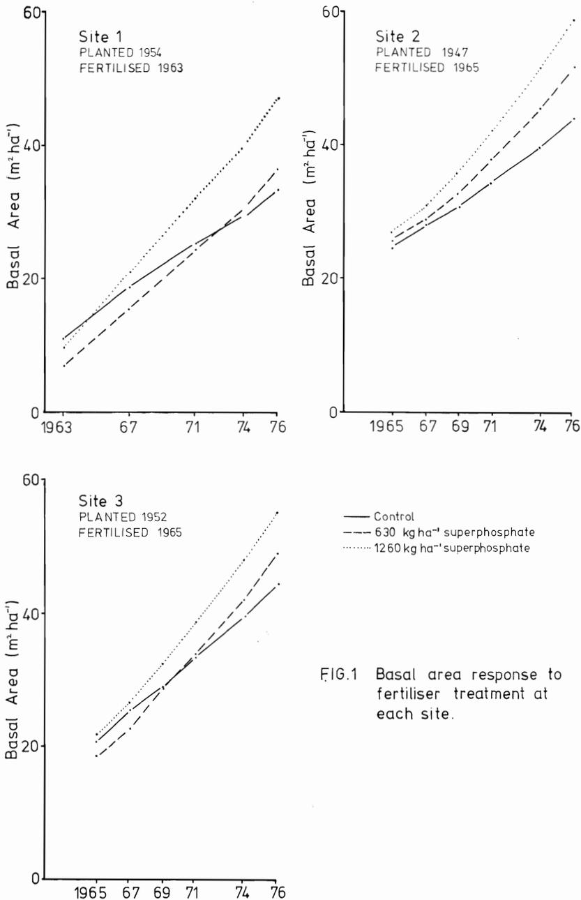
FIG.1 Basal area response to fertiliser treatment at each site.
