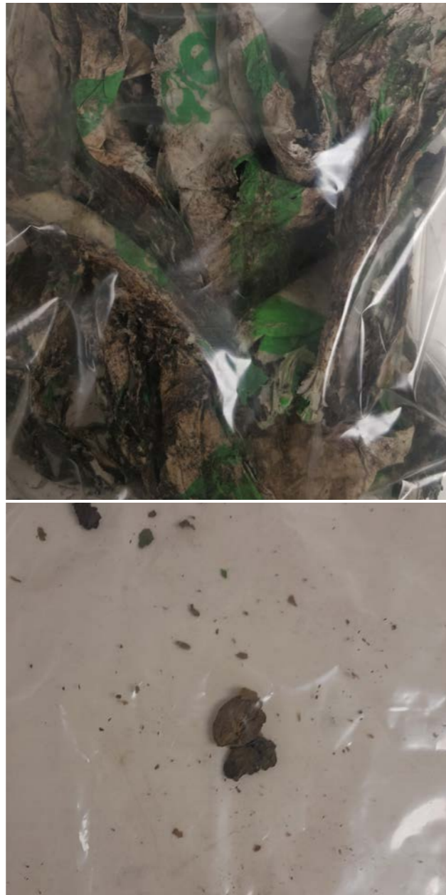
Image 3: Comparison of disintegrated material 0% disintegrated (top) versus 99% disintegrated (bottom).
