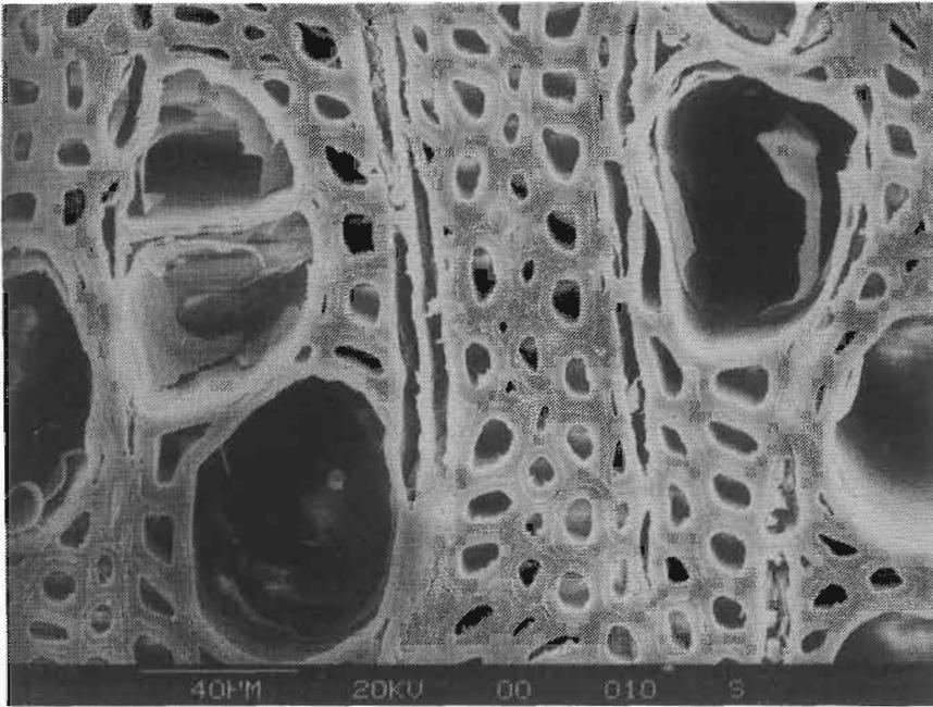
FIG. 4—Ruptured tyloses in *N. fusca* (rolling conditions as in Fig. 2).
