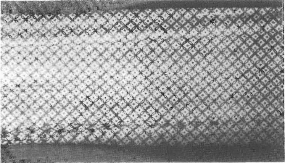
FIG. 5—Deformation of the grid pattern (printed on the edge of a flat-sawn board) while passing out from between the rollers (rolling conditions as in Fig. 3). The compression of the wood is not uniform but is concentrated in the region adjacent to the rollers, where there is extensive localised collapse associated with earlywood of low compressive strength.
