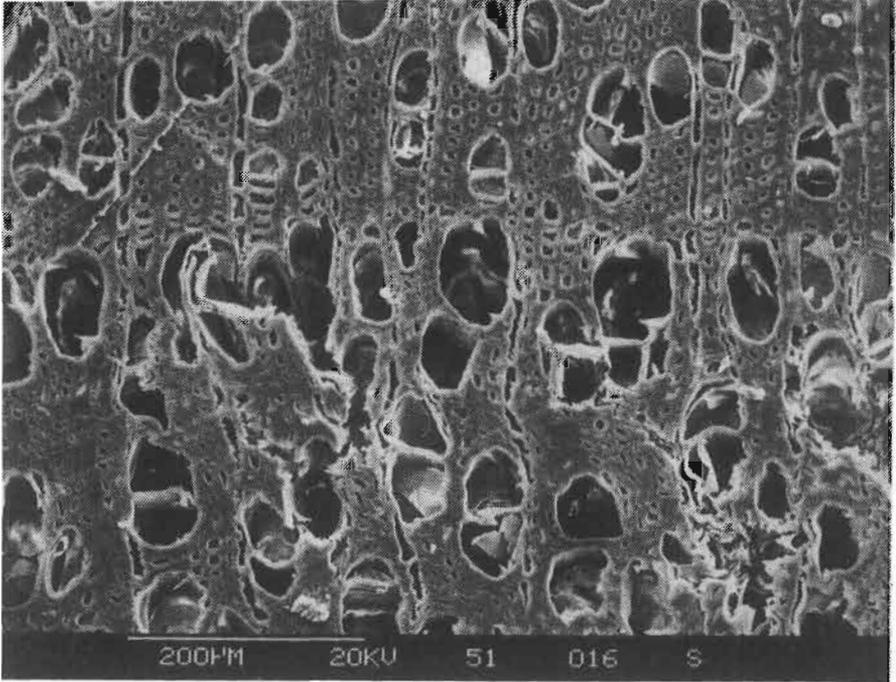
FIG. 2—*Nothofagus fusca* with severely damaged earlywood vessels as a result of rolling green wood (c. 120% mc) between 206.8-mm-diameter rollers at 1000 mm/s with 10% compression.
