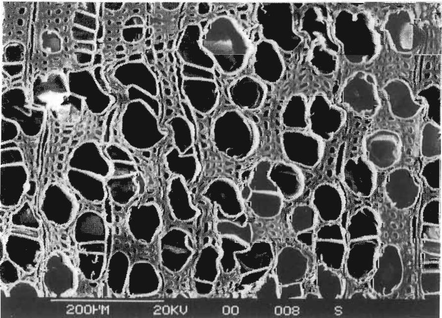
FIG. 3—*Nothofagus fusca* after compression rolling at 20% mc under the same conditions as in Fig. 2.
