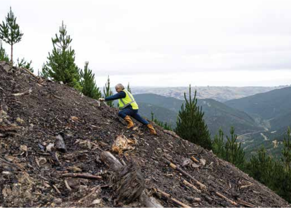
Pushing a 2m long temperature probe into the slash pile at Wenita Forestry, Otago.
