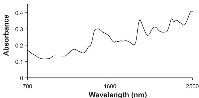
FIG. 2—The average NIR spectrum for the 86 wood specimens.
