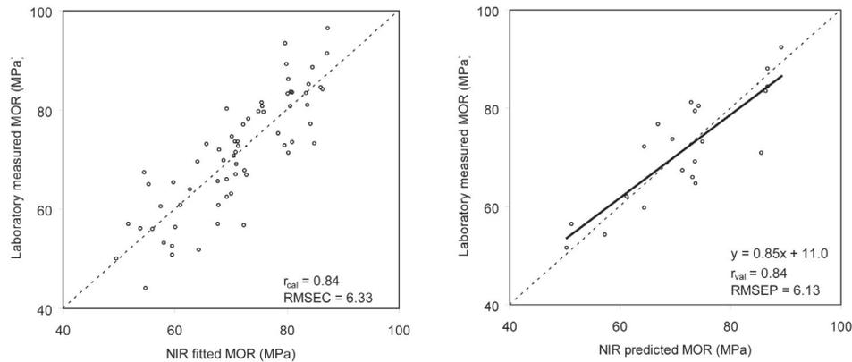
FIG. 5—Results from model calibration (left,  $n = 65$ ) and validation (right,  $n = 21$ ) for modulus of rupture (MOR). The number of partial least squares components is 5. Solid line: regression line for *measured vs. predicted modulus of rupture*; dashed line: target line ( $y = x$ ).
