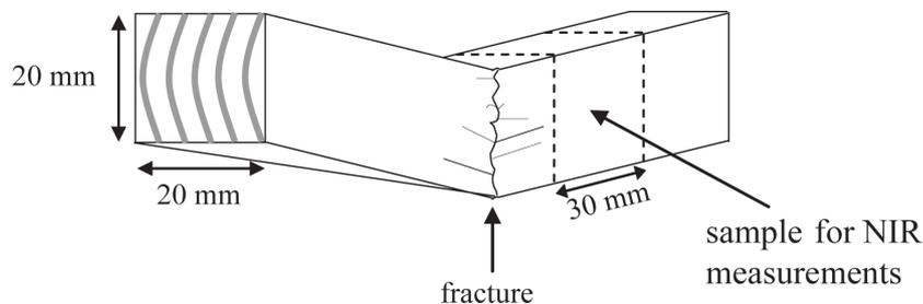
FIG. 1—A wood specimen after modulus of rupture measurements. The sample for NIR measurements is indicated.
