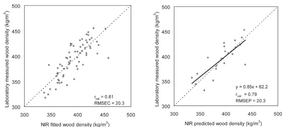
FIG. 3—Results from model calibration (left,  $n = 65$ ) and validation (right,  $n = 21$ ) for wood density. The number of partial least squares components is 3. Solid line: regression line for *measured vs. predicted wood density*; dashed line: target line ( $y = x$ ).
