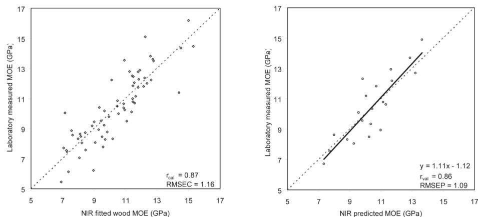
FIG. 4—Results from model calibration (left,  $n = 65$ ) and validation (right,  $n = 21$ ) for modulus of elasticity (MOE). The number of partial least squares components is 7. Solid line: regression line for *measured vs predicted modulus of elasticity*; dashed line: target line ( $y = x$ ).
