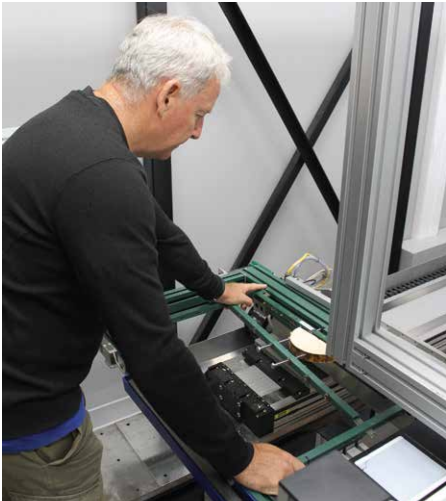
John Lee sets a wood disc into the DiscBot for testing.
