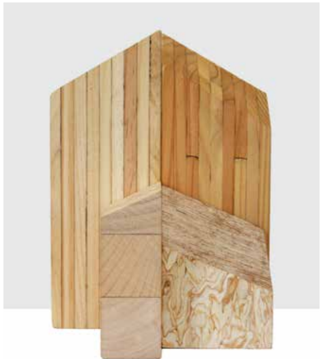
Front left – laminated timber; front right – oriented strandboard (OSB™); rear – oriented engineered laminate (OEL™), a patented technology that uses thin strips of finger-jointed wood laminated together.
