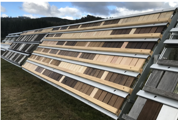
Thermally modified flat panel tests after installation.
