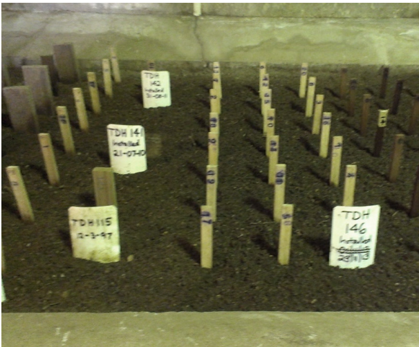
Fungus cellar stakelet testing involves putting sticks into warm, moist soil to accelerate degradation.
