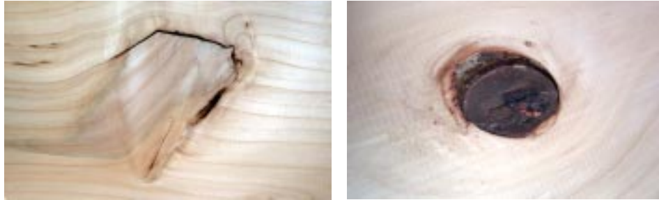
FIG. 2—Leyland cypress. Left : Pruned branch stub, showing absence of intergrowth around dead branch wood (appearing as a dark line). Right : The “stub hole” that results from branch death after pruning and lack of connection to the surrounding wood. The dark resinous material is the dark line in the photo at left.
