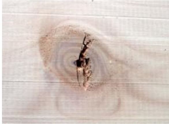
FIG. 1— Cupressus lusitanica : Knot check caused by chipping out during dressing.
