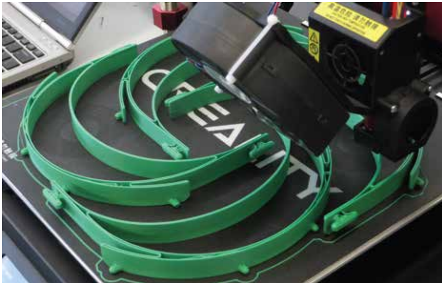
Our additive manufacturing lab became a hive of activity while hundreds of face shield head bands were printed for Lakes District Health Board.
