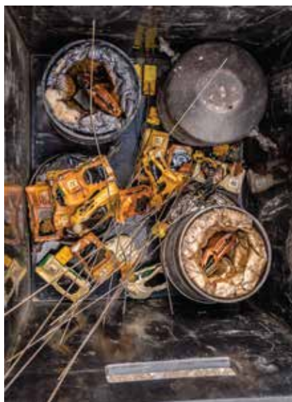
Data loggers recording the rate of fire spread succumb to the heat despite being housed in well-insulated, low-to-the-ground, capsules.
